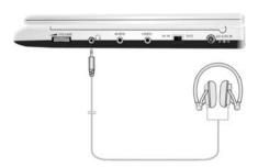
When a headphone is connected, the speakers will automatically turn off.
